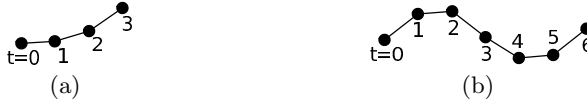
Fig. 2. Action envelopes. New nodes' coordinates are set according to functions of t . In (a), x is linear, y is exponential; in (b), x is linear, y is sinusoidal.
