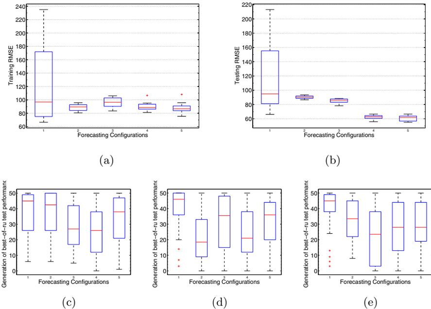
**Fig. 1.** Distribution of best-of-run training and test RMSE accrued from 50 independent runs. Figures (a), (b) for DFW. Figures (c), (d), (e) show the distribution of generation number where each best-of-run individual on test data was discovered for the cases of ATL, DEN, and DFW respectively.
