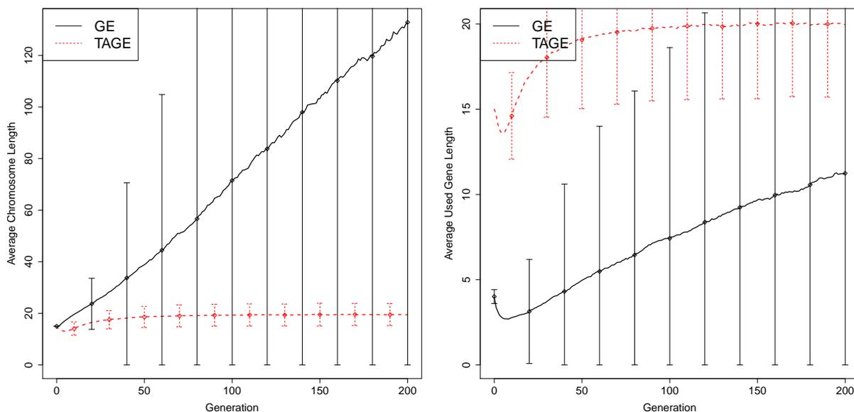
Figure 6.8: Mean chromosome length (left) and mean effective chromosome length (right) plots for GE derivation and TAGE derived trees for the quartic symbolic regression problem with error bars of one standard deviation. The mean chromosome length and mean effective length plots for all problems are provided in Figure B.5 and Figure B.6 respectively.
