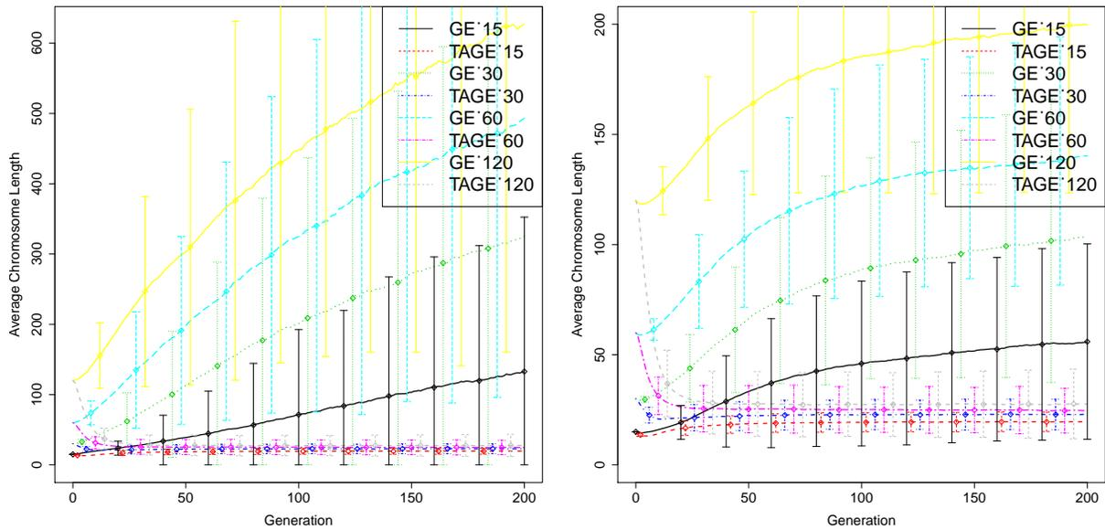
Figure 6.11: Mean chromosome length with no restriction on crossover points (left) and with only encoding region crossover points (right) plots for GE and TAGE for the quartic symbolic regression problem with error bars of one standard deviation. The mean best fitness and mean chromosome length plots for all problems are provided in Figure B.14 and Figure B.15 respectively.
