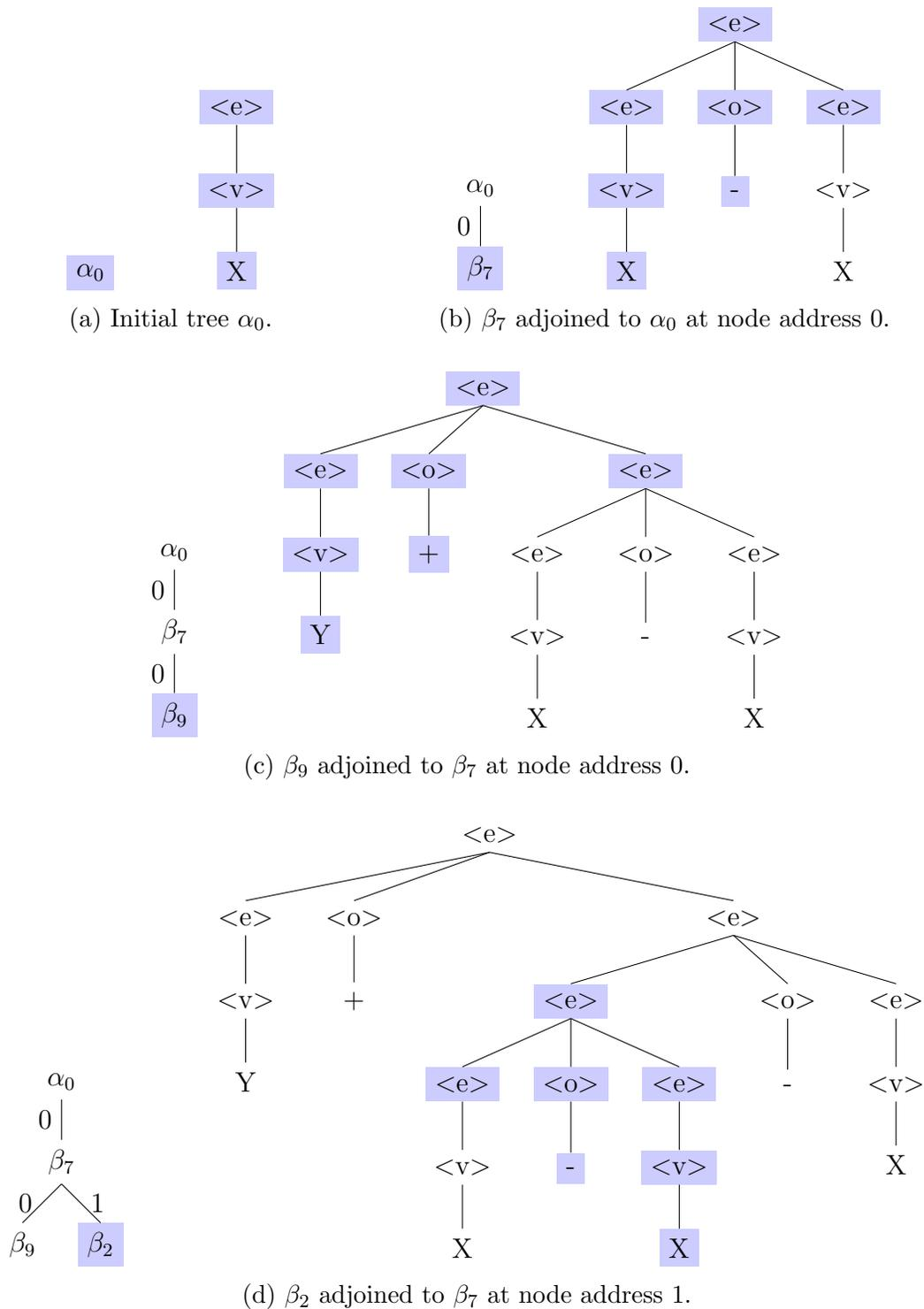
Figure 5.2: The derivation tree (left) and derived tree (right) throughout TAGE derivation. The shaded nodes indicate new content added at each step.
