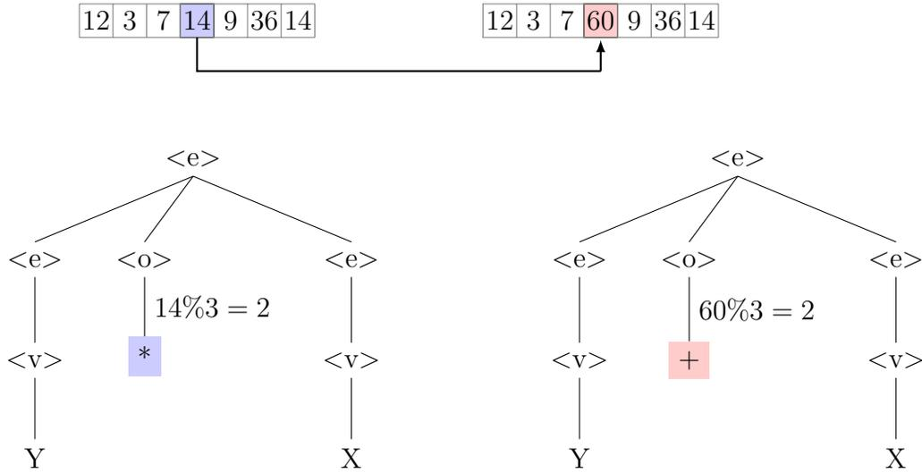
(a) Mutation event where the mutated codon encodes a single terminal node. As the non-terminal nodes in the tree are unaffected no ripple effect is observed. The new phenotype is: Y + X.
