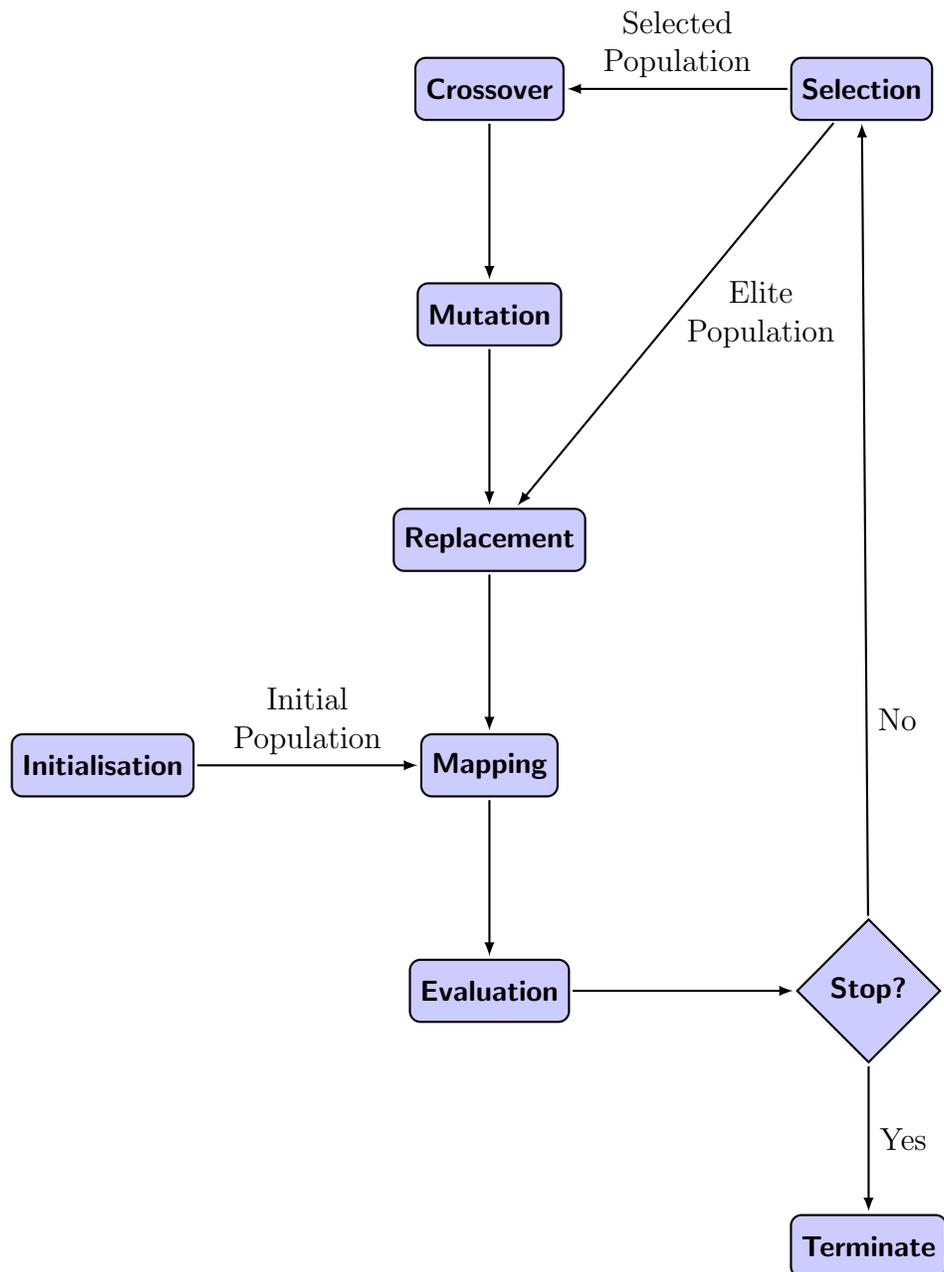
Figure 2.4: The component flow graph of the GE Algorithm.
