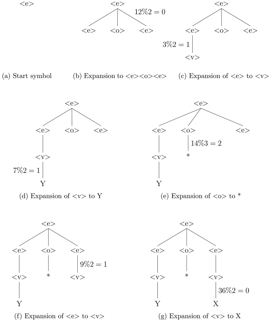
Figure 2.5: An example derivation sequence created from the grammar and chromosome in Figure 2.2. The sub-figures show the derivation tree at each stage of derivation. This results in the phenotype, Y \* X, which is extracted from the leaf nodes of the complete derivation tree.
