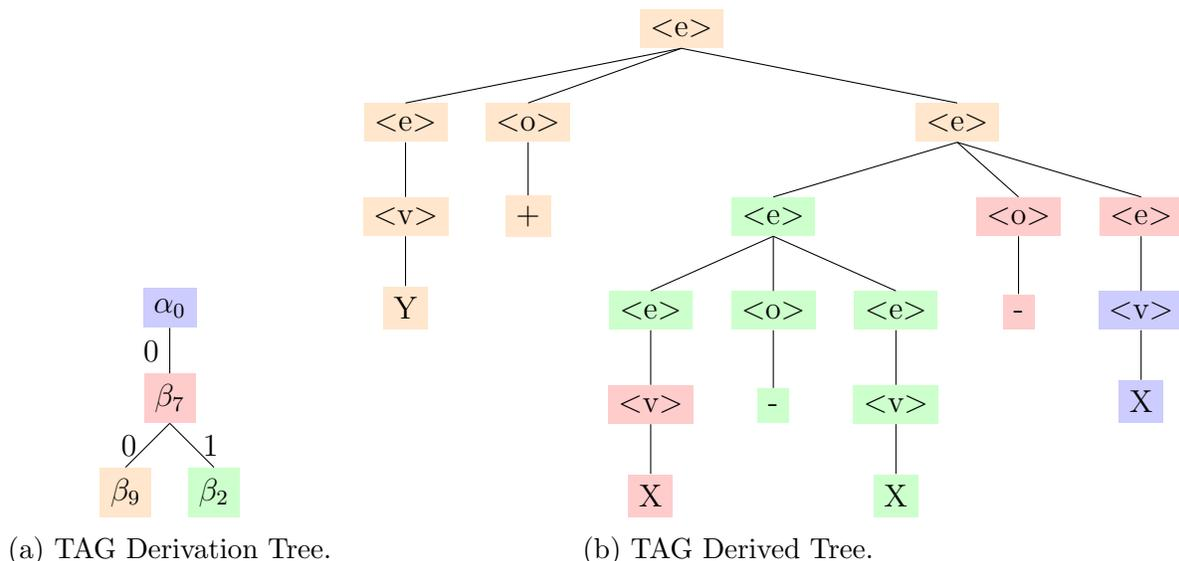
Figure 8.11: An example of a TAG derivation tree and its respective derived tree. Adjunction restrictions can result in the promotion of unbalanced tree shapes.
