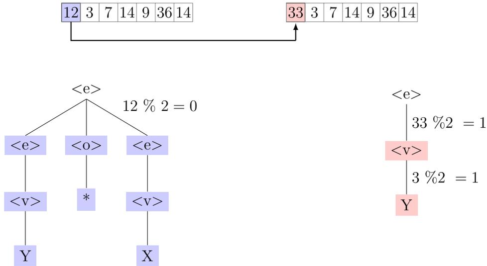
(b) Mutation event where the entire tree is dependent on the selected codon. This causes a ripple effect in the tree, as all codons following the mutated codon are effected and a different tree is derived. This highlights the high linear dependence can be inherent to GE chromosomes. The new phenotype is, Y.
