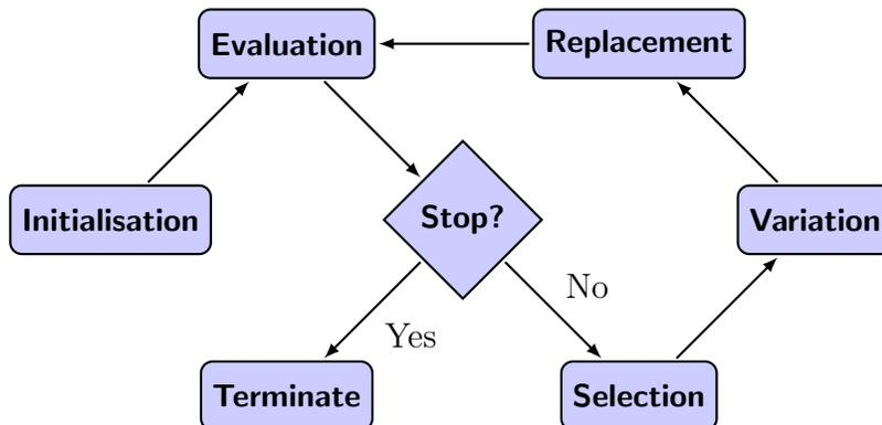
Figure 1.1: Execution flow of a typical EC algorithm.
