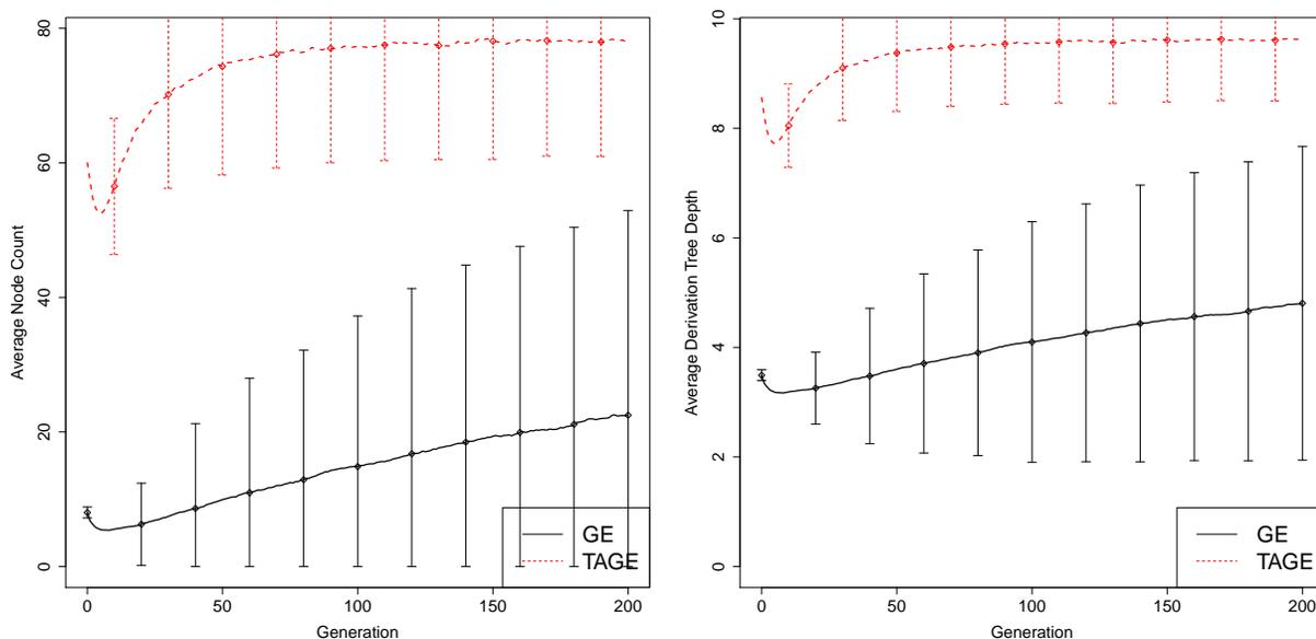
Figure 6.7: Mean node count (left) and mean tree depth (right) plots for GE derivation trees and TAGE derived trees for the quartic symbolic regression problem with error bars of one standard deviation. The node count and depth plots for all problems are provided in Figure B.7 and Figure B.8 respectively.
